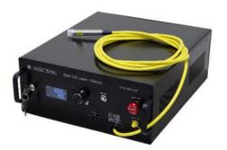
The FCMH series diode lasers deliver up to 500 W of power through a  $200 \,\mu m$  fiber. They provide high brightness and simplified thermal management by distributing the diodes (heat sources), allowing for a water-cooled architecture with reliable, predictable performance. A turn-key benchtop unit is available, integrating the power supply, water cooling, power control, and safety shut-off features.
